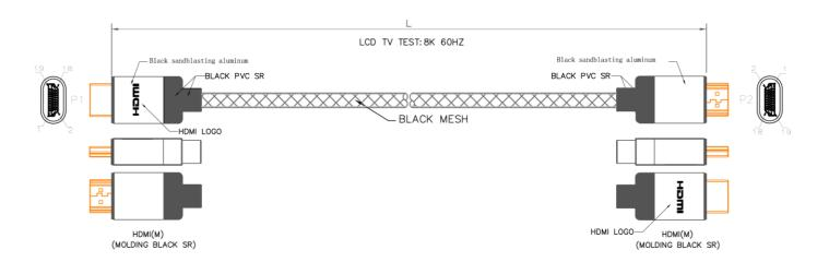
NOTE: E314459  $\,\%$  AWM 20276 80  $^\circ$ C 30V VW-1 HIGH SPEED HDMI  $^\circ$ CABLE WITH ETHERNET
