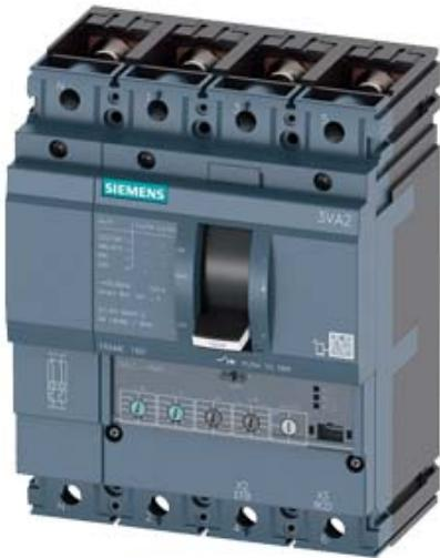
CIRCUIT BREAKER 3VA2 IEC FRAME 160 BREAKING CAPACITY CLASS L ICU=150KA @ 415 V 4POLE, LINE PROTECTION ETU330, LIG, IN=40A OVERLOAD PROTECTION IR=16A ...40A SHORT CIRCUIT PROTECTION II=1,5...12 X IN NEUTRAL PROTECTION ADJUSTABLE(OFF,100%) GROUNDFAULTPROTECTION IG=0,2... 1 X IN, TG=0,1/0,3MS BUSBAR CONNECTION
