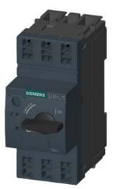
CIRCUIT-BREAKER SZ S00, FOR MOTOR PROTECTION, CLASS 10, A-RELEASE 3.5...5A, N-RELEASE 65A, SPRING-L. CONNECTION, STANDARD SW. CAPACITY
